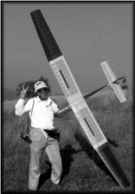
John Vennerholm with Paragon after 8 hour, 2 minute LSF Level V flight. Note waist pack for external transmitter batteries. Blue and yellow transparent monokote gave excellent, high altitude visibility.
